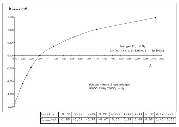
Note: these characteristics are valid for the specified test gas only. They may be different for real engine exhaust gas and must be determined separately.
