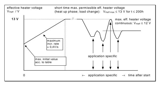
Maximum permissible heat up rate with limited heater power to reduce the thermal stresses in the heat-up phase
